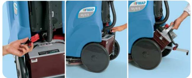
The battery - when flat - can be easily replaced with a new one so that the machine provides longer operating cycles.
